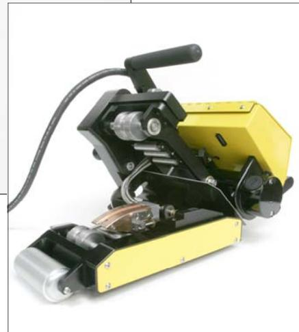
The wedge assembly can be **removed in 30 seconds** by simply unplugging the external heater and thermocouple plug-in wire connector, removing two shoulder bolts, and opening up the frames as shown above. Just lift the wedge assembly and pull it out!
